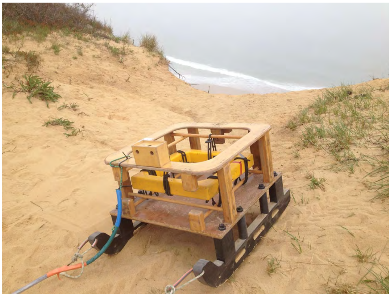
Figure 5 – TDEM Receiver Antenna, East End of Route A
